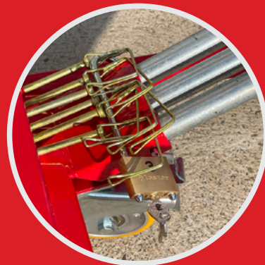
Lockable storage for poles and shaft lock pins
